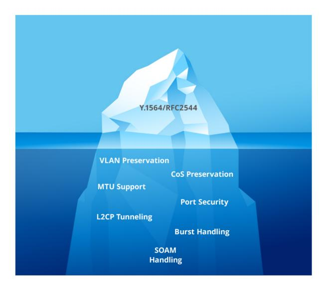
Often Carrier Ethernet Service Providers Rely On Either Itu-T Y.1564 Or Rfc2544 Tests, To Check Network Integrity Before Service Turn-Up. As The First Part Of The Article Described, That Much Like The Proverbial "Tip Of The Iceberg", There Are A Number Of Other Problems That Could Potentially Lie Undetected Until Customers Start Using The Network.
