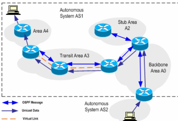
Figure 1: Example autonomous network supporting OSPF3 functionality
